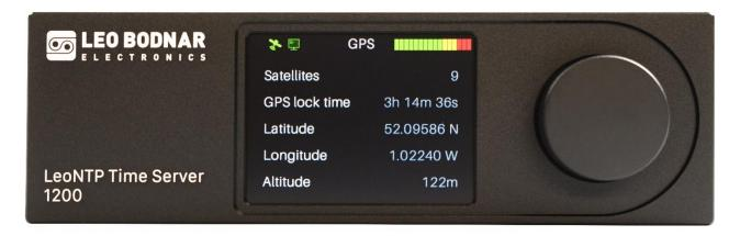
This screen shows the current time the unit has been locked, the satellites and current location. There is nothing to configure under this screen and is for information only.
