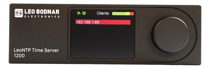
This screen shows the current NTP clients that are currently connecting to your device. Red means more than one connection a second. There is nothing to configure under this screen and is for information only.
