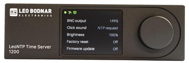
This screen lets you view or select the BNC output, the behaviour of the clicker, screen brightness, factory reset and Firmware Upgrade options.
