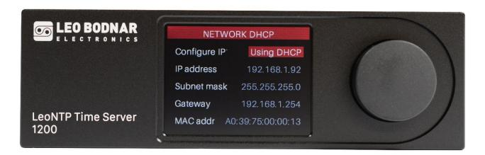
The IP address settings in manual mode can be set by rotating left and right to select the value of each octet. Press the button to move to the next field. Subnet mask and gateway are set in the same manner. Settings are immediate and the unit doesn't need a reboot.
